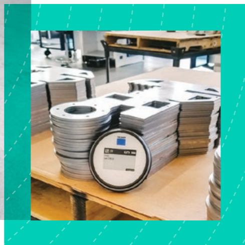
Track&Trace: Satellites and markers increase the transparency on a shop floor
